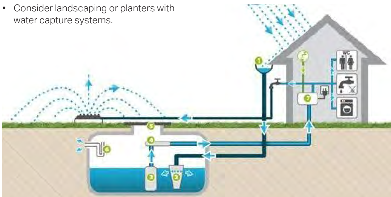
Figure 89: Diagram illustrating rainwater harvesting systems that could be integrated into open space and residential developments. Source: https://dps-fr.com/
