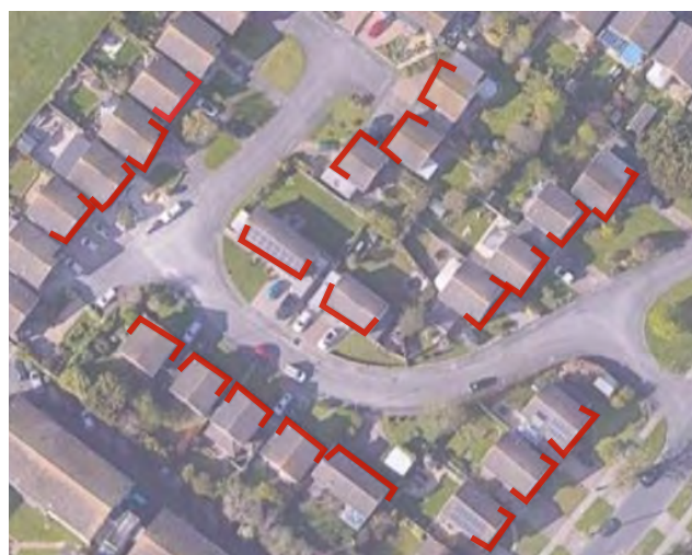
Figure 59: Areas of cul-de-sacs are typically narrower and have consistent building lines that follow gently meandering streets. Smaller degrees of building setback and varied building orientations result in a less formal pattern of development with a stronger sense of enclosure, Loos Barn Close.
